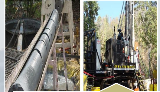
Large Diameter Kimberlite core (8") for Rio Tinto at Bunder, MP – Drilled by BLY LF230 upto a depth of 352 Meters. largest coring done in India till date
